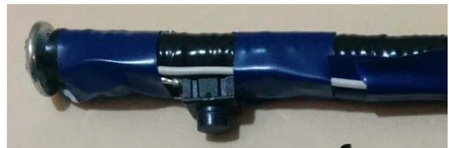
Figure 2. Push button to turn the electromagnet on or off
